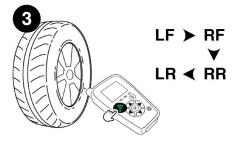
Trigger each sensor around the vehicle, in the listed order, pressing the green trigger button at each sensor.
