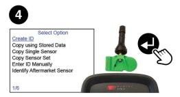
From the Program menu, Select Create ID. Once on the next screen, place the sensor in front of the tool and press the enter button.
