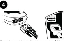
Turn the vehicle's ignition to the ON position, and connect the OBDII cable to the tool and the other end to the vehicle.
