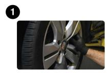
Before performing a relearn, ensure the new sensor(s) are properly installed, and the wheel(s) have been put back on.
